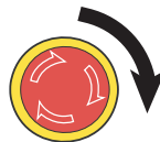
Fig. 1-4: Release of emergency stop button by turning
